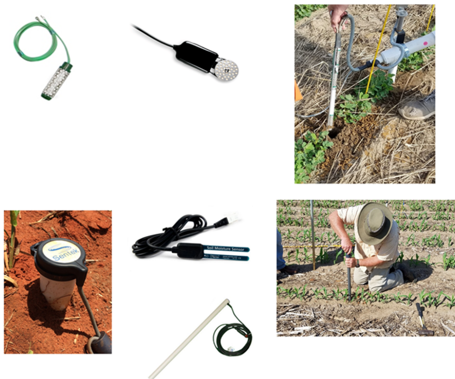
Figure 7: Sensor-based system, including tensiometric sensors (top) and capacitance sensors (bottom).
